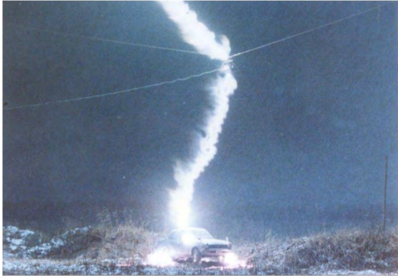
Triggered lightning strike to car with live rabbit inside (Japan). The rabbit was unharmed. Notice current arcing to ground from hubs.
